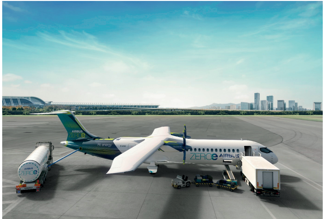
Figure 1 Airbus ZEROe turboprop concept with visible refueller on the left side Copyright: Airbus 2023
