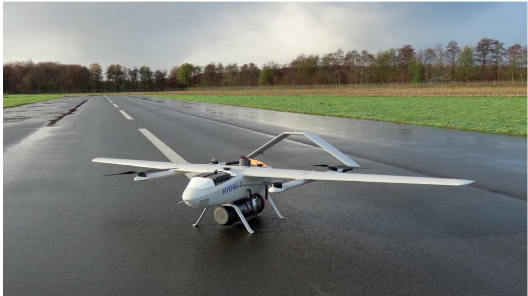
Figure 5 The LH 2 -powered HYDRA 2 drone
