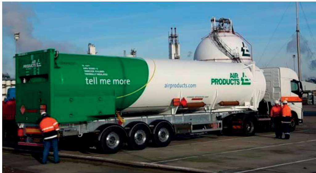
Figure 10 LH 2 trailer from Air Products Source: Air Products
